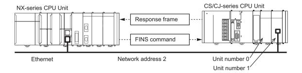
The example below shows the routing table setting for the NX-series CPU Unit.
