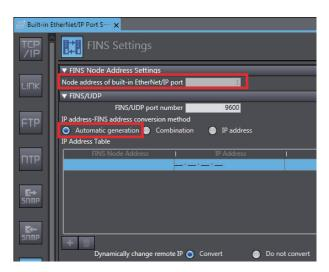
When the combination or IP address method is selected, the value specified for the FINS node address settings is used as the FINS node address.
