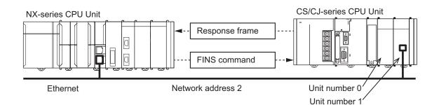
The example below shows the routing table setting for the NX-series CPU Unit.
