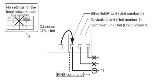
\*1. When the FINS command specified with network address 0 and node address n is issued to a CPU Unit with no local network table specified, the FINS command is issued to the FINS network of the lowest unit number.
