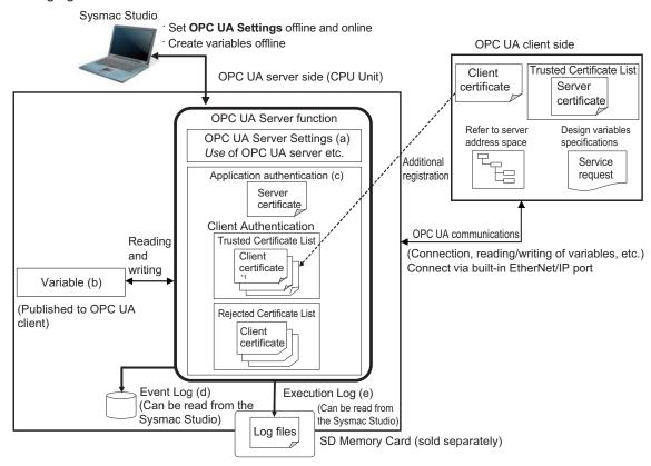
Note The above figure shows the case of a self-signed client certificate.
