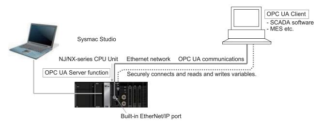
Refer to *A-6 Version Information* on page A-27 for the unit version of the CPU Unit and the version of the Sysmac Studio that can be supported.
