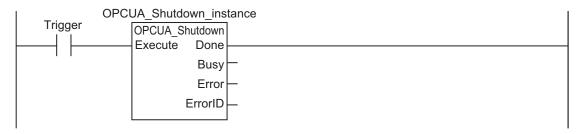
When the instruction is normally completed, the Shutdown\_OK variable is changed to TRUE.
