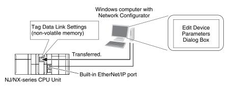
For details on the Network Configurator, refer to *Section 6 Tag Data Link Functions* on page 6-1.
