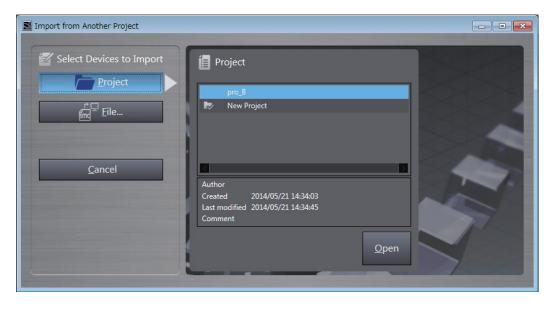
The list of EtherNet/IP devices registered in the selected project will be displayed. Select the target devices to import, and click the **Import** Button.
