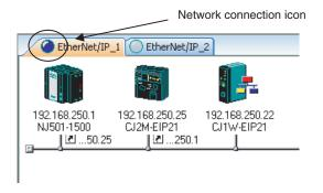
Select Network - Change Connect Network to switch the connected network.
