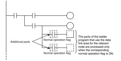
• The following shows an example where data processing is performed only when data links are operating normally with MC and MCR instructions, or with JMP instructions.
