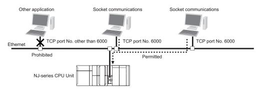
Packet Filter settings are as follows: For Protocol, tcp is selected and 6000 for the source port.
