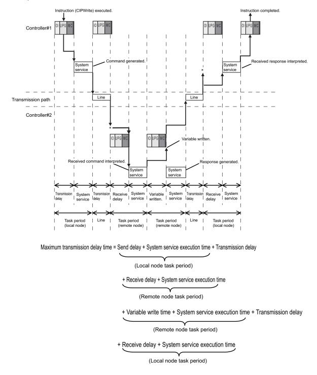
Processes with delay time are processed within the task period of each node as shown in the above diagram.
