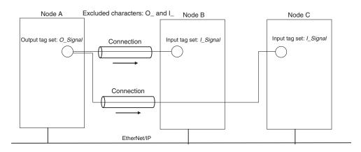
**1** Set the same tag set names for the output and input tag sets for the connection. The tag set names can also include forward and backward ellipses.
