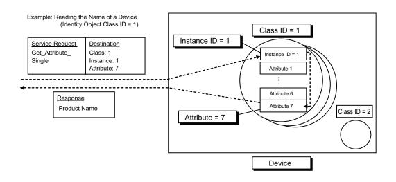
These are called *IOI* (Internal Object Identifier) because they identify the Class ID, Instance ID, and Attribute ID within the device.
