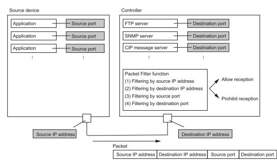
Packet Filter function can enable or disable the reception of packets using these four types of information. If the content of the packet matches the permitted content in Packet Filter settings, reception is permitted. Otherwise, reception is disabled and the packet is discarded.
