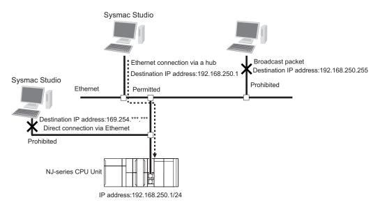
Packet Filter settings are as follows. Set the IP address for the Controller's built-in EtherNet/IP port to the destination IP address.
