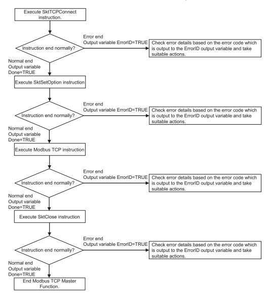
If the response from the other equipment is slow and the Modbus TCP instruction ends before the response is returned, there may be data remaining in the receive buffer. In such cases, execute the Modbus TCP instruction after the receive buffer is cleared with the SktClearBuf instruction or SktTCPConnect instruction.
