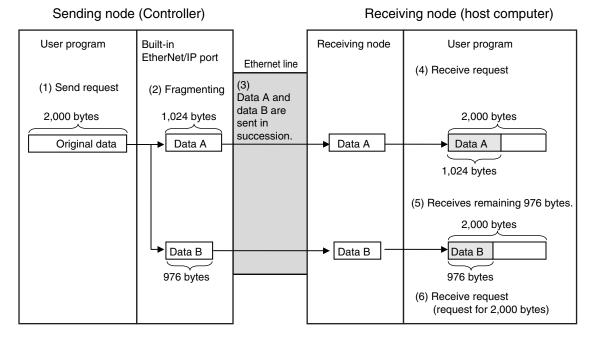
Data is delivered to the user program in a fragmented form in TCP communications, as shown above.
