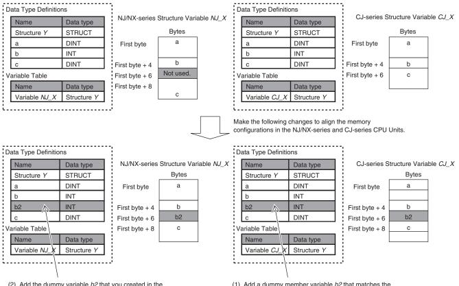
(2) Add the dummy variable b2 that you created in the CJ-series CPU Unit to the NJ/NX-series CPU Unit as well. (1) Add a dummy member variable *b2* that matches the unused memory location on the NJ/NX-series CPU Unit.
