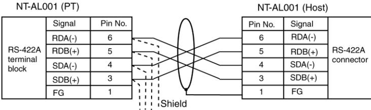
● **Wiring Layout between NT-AL001 and NT-AL001 (RS-422A)**
