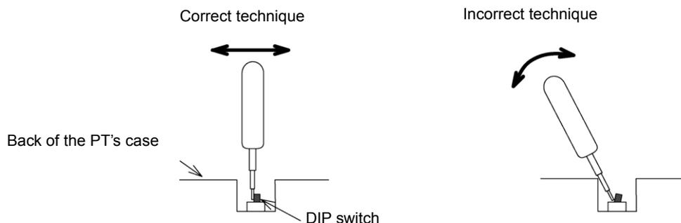
The DIP switch may bend or break if the tool is incorrectly levered against the PT's case as shown in the diagram.
