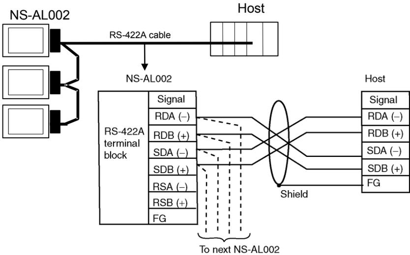
When connecting individual signals with twisted-pair cable, connect RDA and RDB, and SDA and SDB, as pairs in the twisted-pair cable. A communications error may occur if the pairs are not combined correctly.
