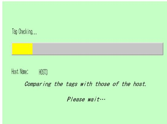
2. When verification has been completed, the user screen will be displayed if the tags of the NS-series PT and the host match.
