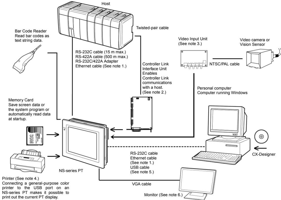
Note 1: Only the following models support Ethernet: NS15-TX01□-V2, NS12-TS01(B)-V□, NS10-TV01(B)-V□, NS8-TV□1(B)-V□, NS5-SQ□1(B)-V□, NS5-TQ□1(B)-V□, and VS5-MQ□1(B)-V□.
