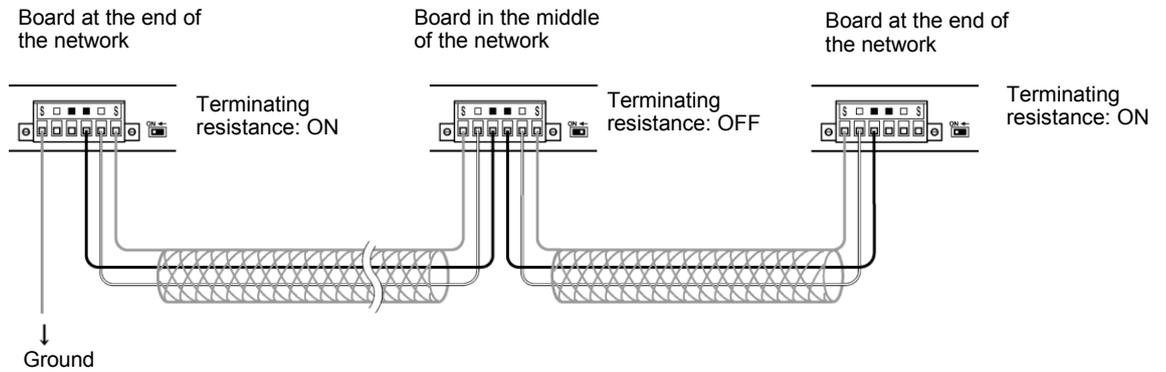
**Reference** • Terminals of the same type are connected internally. They can thus be connected to either the right or left half of the end Boards.
