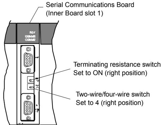
• **Connecting to CVM1/CV Series (-V□) PLCs (Using RS-232C/RS-422A)**
