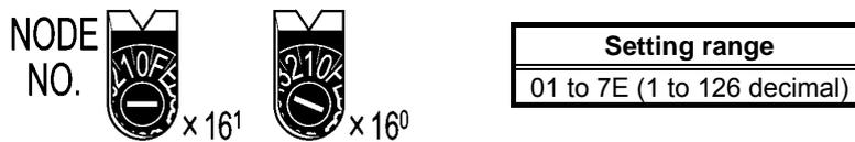
Set the upper digit using the left rotary switch and the lower digit using the right rotary switch.
