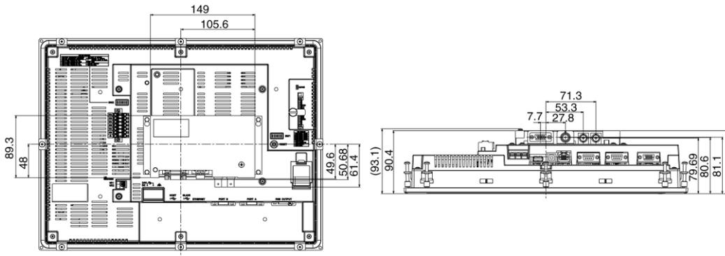
● NS15 Controller Link Interface Unit Mounted Dimensions
