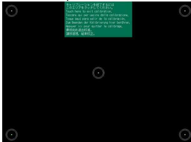
2. Press the marks in the four corners of the screen and the mark in the center of the screen. The marks may be pressed in any order.
