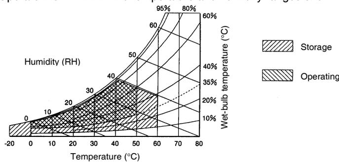
3. When a STN LCD display device is used, the display quality will decline (e.g., the contrast ratio will be reduced) if the temperature exceeds 40°C. Also, when the temperature drops, the response speed is lowered due to characteristics of liquid crystals. This applies to the following models. Refer to *NS-series PT Lot Numbers* on page A-8 for information on lot numbers.
