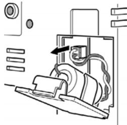
4. Connect the new battery connector, and insert the battery into the battery holder in the battery cover.
