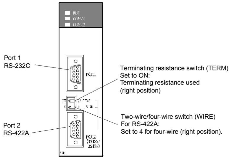
**Connecting to CS-series Serial Communications Units**
