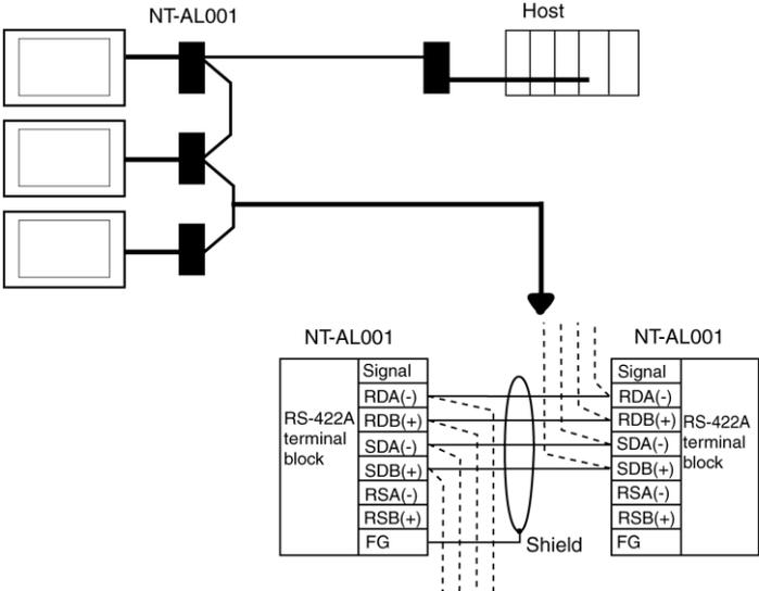
● **Wiring Layout to CS1G/H Serial Communications Boards, C200HX/HG/HE(-Z) Communications Boards, CQM1H Serial Communications Boards, and CVM1/CV Series Host Link Units**
