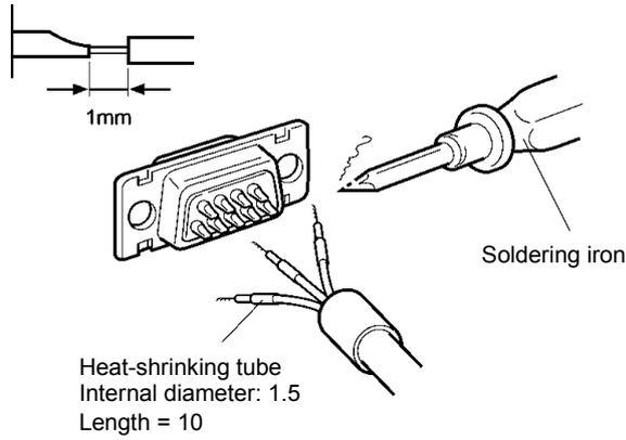
4. Replace the heat-shrinking tube up to the soldered section, and shrink the tube onto the wire by applying heat using a soldering gun.
