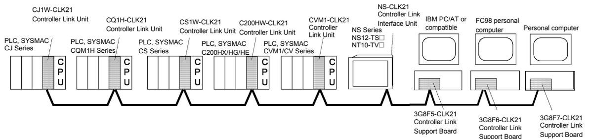
To connect the PT to the Controller Link, it is necessary to install a Controller Link Interface Unit on the PT. A Controller Link Interface Unit can be used only for the NS15, NS12 and NS10 NS-series PTs. Refer to *3-8 Installing the Controller Link Interface Unit* for the procedure for installing and wire the Controller Link Interface Unit.
