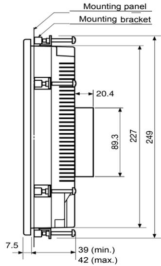
● NS12-V1/-V2, NS10-V1/-V2 Cable Connection Dimensions
