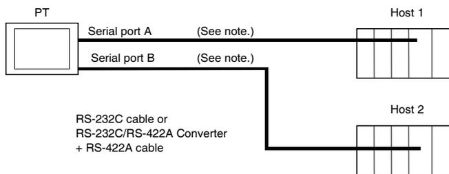
Note: Each port allows 1:N connection. NS-AL002 connects either serial A or serial B, but not both due to structural restrictions.
