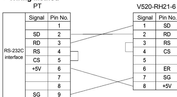
When connecting to the 5-V output of the PT's serial port, use a cable length of less than 2 m. If the cable is 2 m or longer, connect pins 7 and 8 of the Bar Code Reader to an external power supply.
