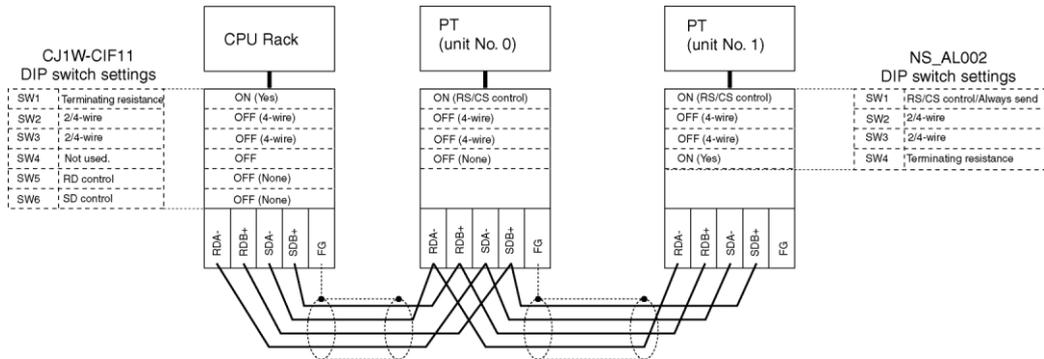
**Note:** Refer to A-3-6 *Handling the Shield on RS-422A/485 Cables* for information on processing the shield wire on the RS-422A/485 cable.
