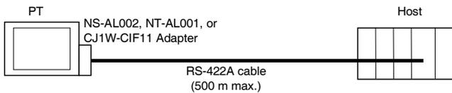
\*1: The maximum transmission distance is 50 m when using the CJ1W-CIF11.
