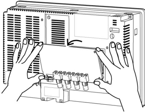
Remove the upper side of the Video Board first, holding the four corners.
