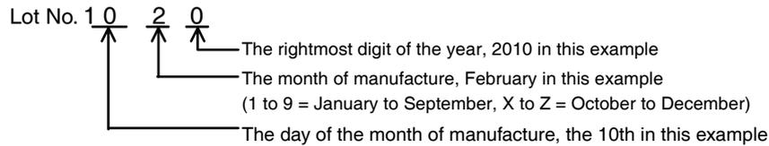
The five-digit lot number that is given on the back of an NS-series PT can be used to check the manufacturing date of PTs that were manufactured on June 1, 2012 or later.
