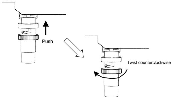
2. After unlocking the BNC socket, pull it out.
