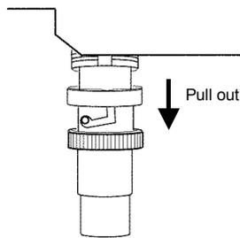
If the camera's video output cable uses an RCA plug, connect it to the video input connector using a BNC-RCA connector in the way shown below.
