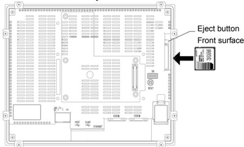
2. Push the Memory Card firmly into the back of the slot. (The eject button will be pushed out when the Memory Card is installed properly.)
