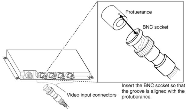
2. After inserting the BNC socket, twist it clockwise until it locks into place.
