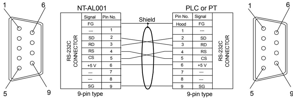
When connected to a PLC with a +5-V output, an external power supply is not required for the NT-AL001.
