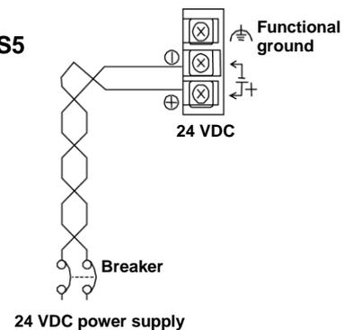
• **Parts Used to Connect the Power Supply**
