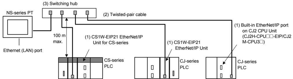
The following devices are required to configure a network using an EtherNet/IP Unit and must be purchased separately. Prepare the devices in advance.
