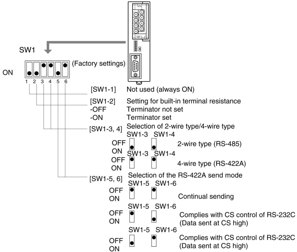
When using the host link or 1:1 NT Link, set the RS-422A send mode to continual sending (set both SW1-5 and 6 OFF).
