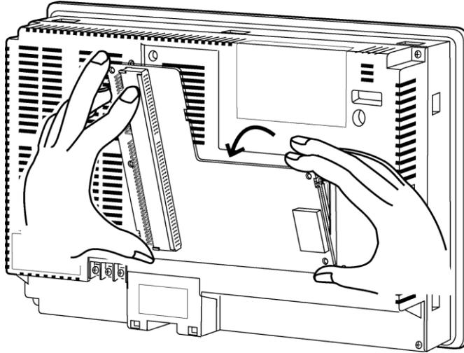
Hold the four corners of the Board and detach upper side first.
