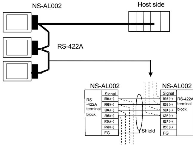
● Wiring Layout between NT-AL001 and Host (RS-422A)
