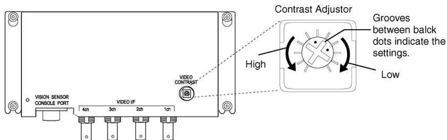
If turning the contrast adjuster too much, the image may be distorted. Turn the contrast adjuster in the opposite direction to remove the noise.
