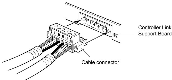
2. Secure the connector to the Board by tightening the screws on the connector. The applicable tightening torque is 0.2 N·m.
