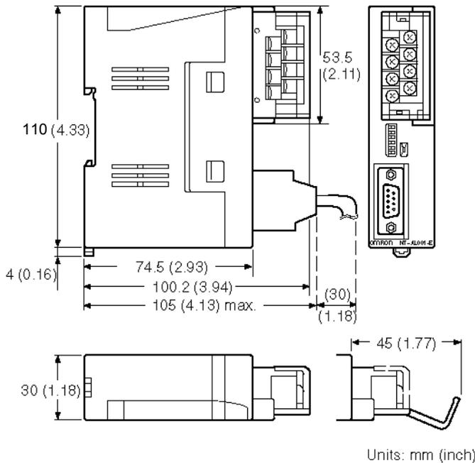
30 (W) × 114 (H) × 100.2 (D) mm: with the RS-422A terminal block cover closed
