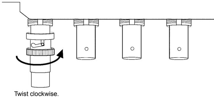
● **Removing the Video Input Connector**
