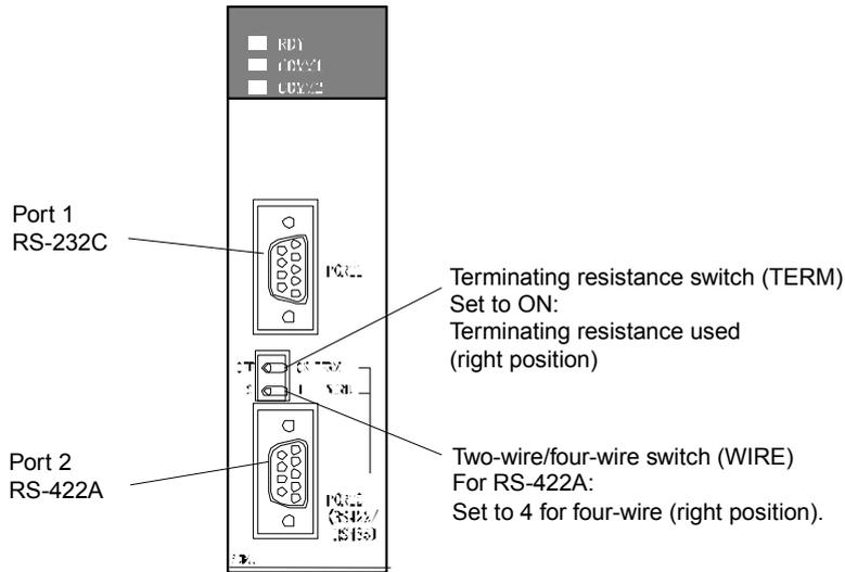
**Connecting to CS-series Serial Communications Units**
