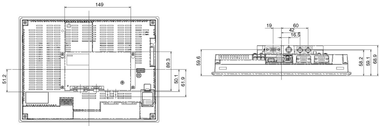
● NS12-V1/-V2 and NS10-V1/-V2 Controller Link Interface Unit Mounted Dimensions
