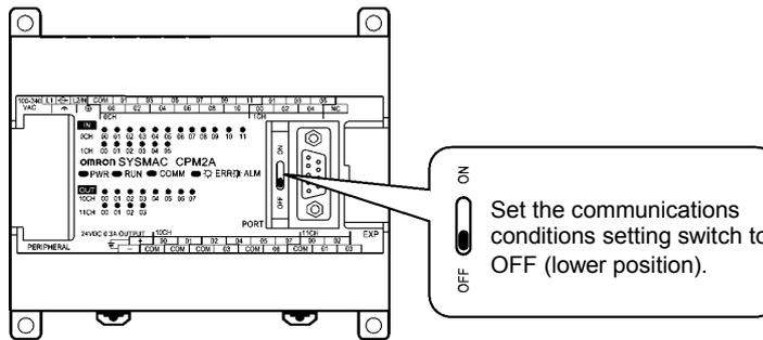
• **Setting the CPM2C Front Panel DIP Switches**
