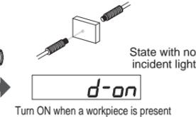
3. Press the [MODE] button for 3 seconds or longer to return to the Detection Mode.
