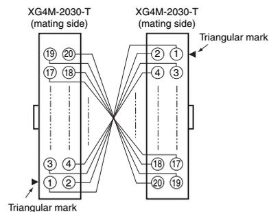
Note: Connector pins are connected 1-to-1 so that pin numbers correspond.
