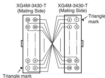
Note: Wire the pins 1:1 so that the Connector pin numbers match.
