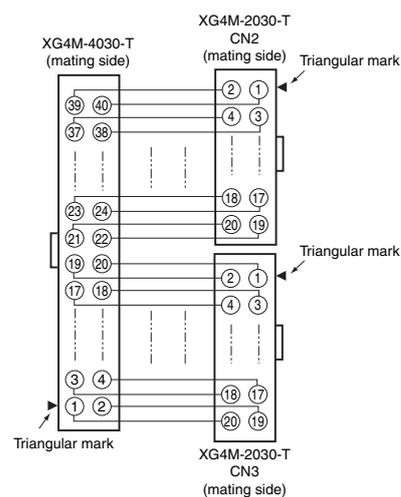
**MIL 20-pin - MIL 20-pin, Straight Wiring**
