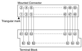
Note: For all models, the odd-numbered pins on the Connector correspond to row A on the terminal block and the even-numbered pins on the Connector correspond to row B on the terminal block.
