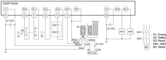
S1: Emergency stop switch S2: Safety door switch (D40A-2)
