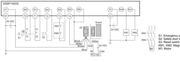
S1: Emergency stop switch S2: Safety door switch (D40A-2)
