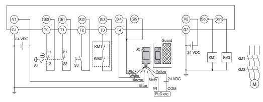
S1: Emergency stop switch S2: Non-contact door switch (D40Z) S3: Reset switch KM1, KM2: Magnetic contactors M: Motor
