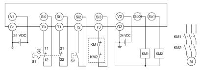
Emergency stop switch Reset switch KM1, KM2: Magnetic contactors Motor
