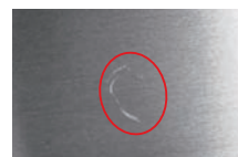
White scratch on shaded hairline finish
