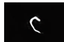
White scratch on shaded hairline finish
