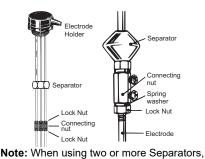
te: When using two or more Separators, be careful with the mounting direction of the connecting nut screws which connect electrodes. Avoid the screws from touching each other.
