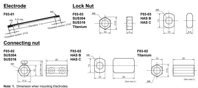
2. Clamp screws are not provided for HAS B, HAS C, or titanium models. F03-03 Lock Nuts are used to mount Electrodes.
